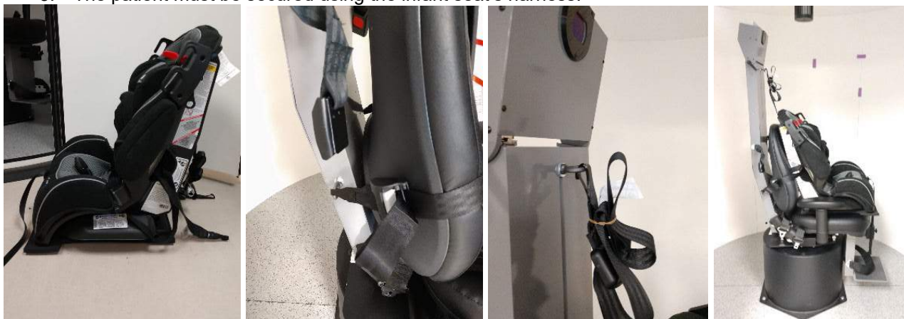
Figure 2.6-29: Sequential images of infant car seat fitting on Auto-Traverse/Comprehensive Chair (left to right)
