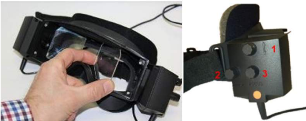
Figure 2.6-4: Adjustable IR mirrors for interpupillary distance adjustment (left), and knobs for 1) vertical camera adjustment, 2) horizontal camera adjustment, 3) camera focus adjustment (right)
