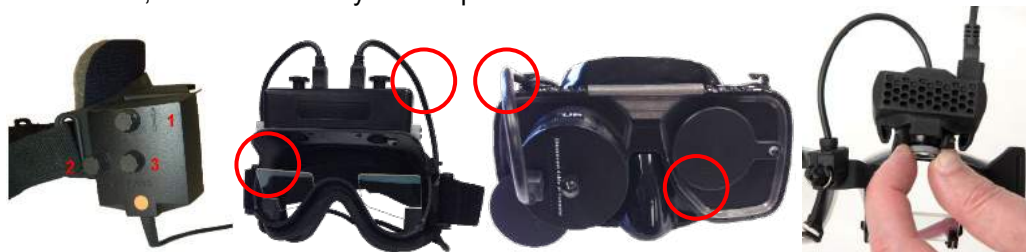
Figure 3.6-2: Focus adjustment on the different VNG and vHIT goggles
