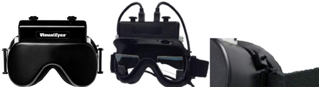
Figure 2.6-5: Top mount goggle with cover (left), without cover (middle), and start/stop switch on goggle (right)
