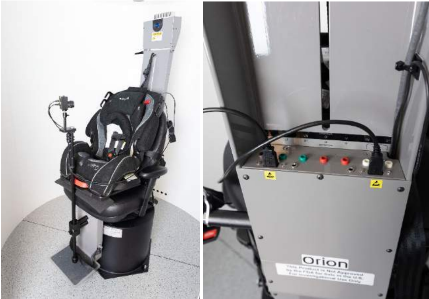
Figure 2.6-30: Pediatric observation camera attached to the Orion Auto-Traverse/Comprehensive chair and connected to the USB ports on the back of the chair
