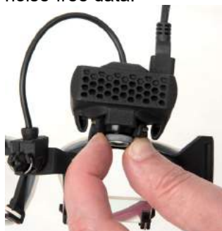
Figure 2.6-8: Focus adjustment on the EyeSeeCam goggle
