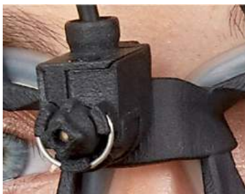
Figure 2.6-9: Calibration laser on the EyeSeeCam goggle.
