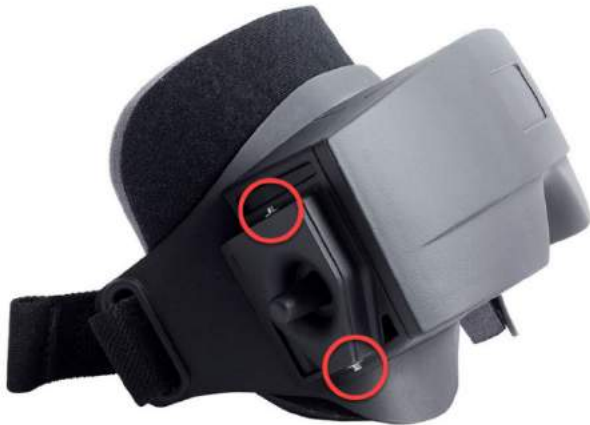
Figure 2.6-3: Hexagon fixation screws on the top and bottom of the side mount goggle, used for fixation of a camera or fixation of a cover (in picture)
