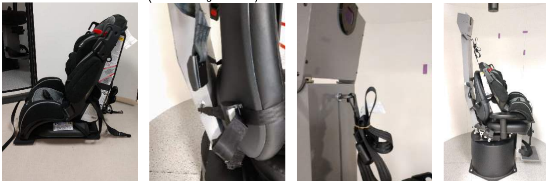
Figure 3.5-4 Sequential images of infant car seat fitting on AT/C Chair (left to right)
