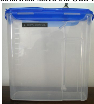
Figure 4 External tank with pick up filter
