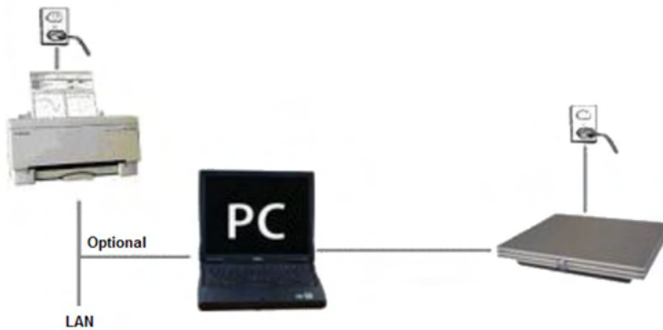
Fig.2: Eclipse is powered from mains and is connected to a computer via USB cable. The computer can be attached to other devices and still maintain patient safety.
