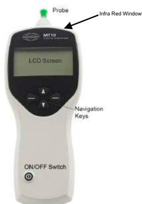
The function of the left and right keys is usually shown on the bottom line of the display. When not performing a test the MT10 will switch off automatically if no key is pressed for 90 seconds. This time can be extended to 180 seconds in the CONFIGURATION menu.
