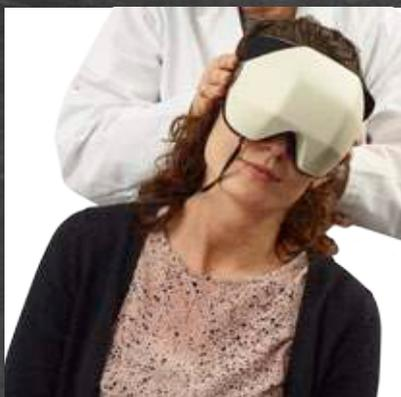
The goggles are fitted with movement sensors to allow for SVV testing to be performed at multiple static tilt angles.
