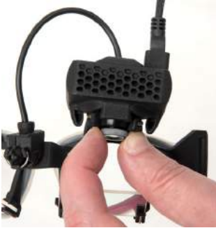
图 2.6-8: EyeSeeCam 眼罩的焦距调节
