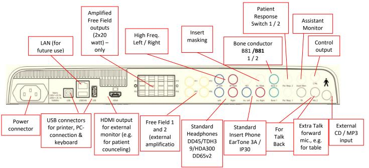
The back panel contains all the rest of the main connectors (sockets):
