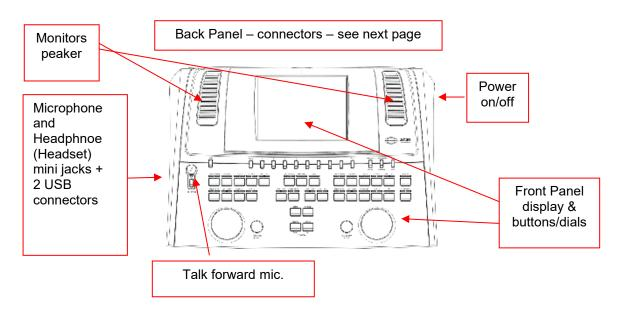
The top left part of the AC40 (display holder) contains the two monitor speakers.
