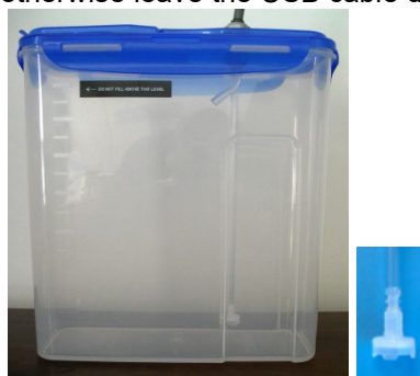
Figure 4 External tank with pick up filter
