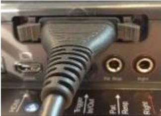
1. Locate the probe connection on the back of the unit.
