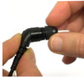
Step 1: Unscrew the probe cap and remove the probe tip.
