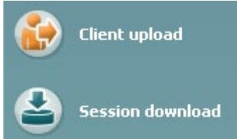
**Client upload** is used for uploading clients from the database (Noah or OtoAccess®) to the AT235. The internal AT235 memory can hold up to 500 clients and 50.000 sessions.
