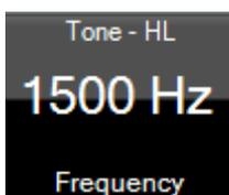
C The measurement type (HL, MCL, UCL or Tinnitus is shown) as well as the presentation type (tone or pediatric noise) and the test frequency is shown.
