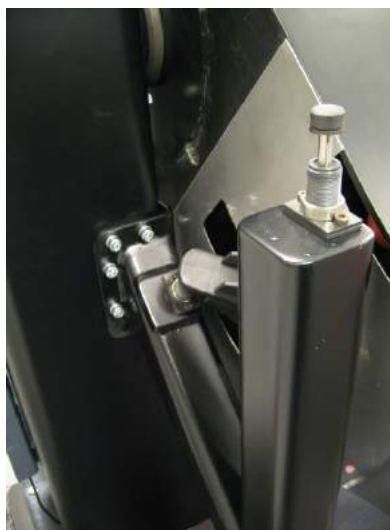
Stop will engage with lower hydraulic shock absorber during vertical canal DPRM.
