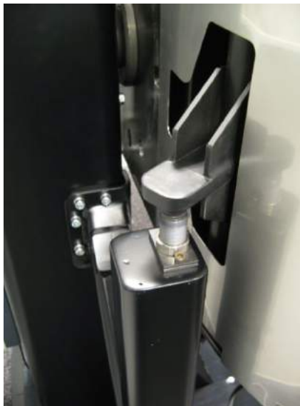
Stop will engage with upper hydraulic shock absorber during horizontal canal DPRM.
