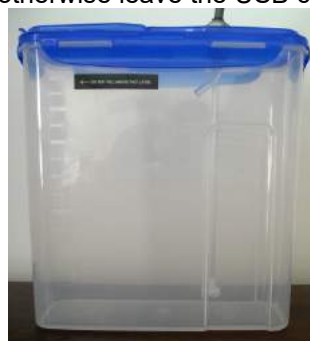
Figure 4 External tank with pick up filter
