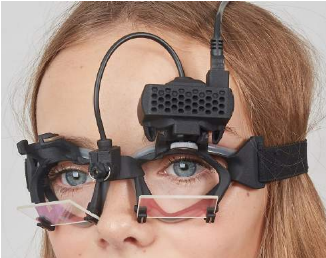
Figure 3.3.1-1vHIT goggle and ball and socket joint for camera. Calibration laser is placed on the bridge of the goggle.
