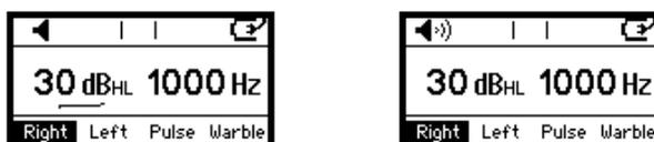
B) **Response:** When using the APS3 response button, a response is indicated in the middle of display header.
