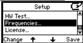
Press Change to access the default frequency range from 125Hz to 8 kHz for daily operation.
