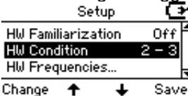
Press Change to toggle between “2 correct out of 3 answers” and “3 correct out of 5 answers”. The conditions used before going to the next frequency.
