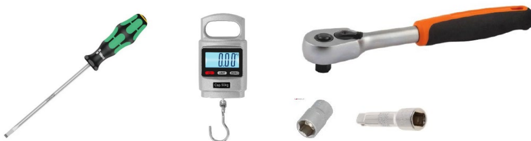
Figure 35: Tools needed to adjust drive belt tension
