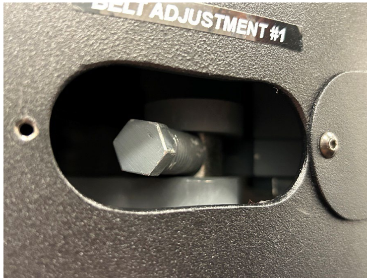
Figure 38: Adjustment bolt at entry point for Belt #1.
