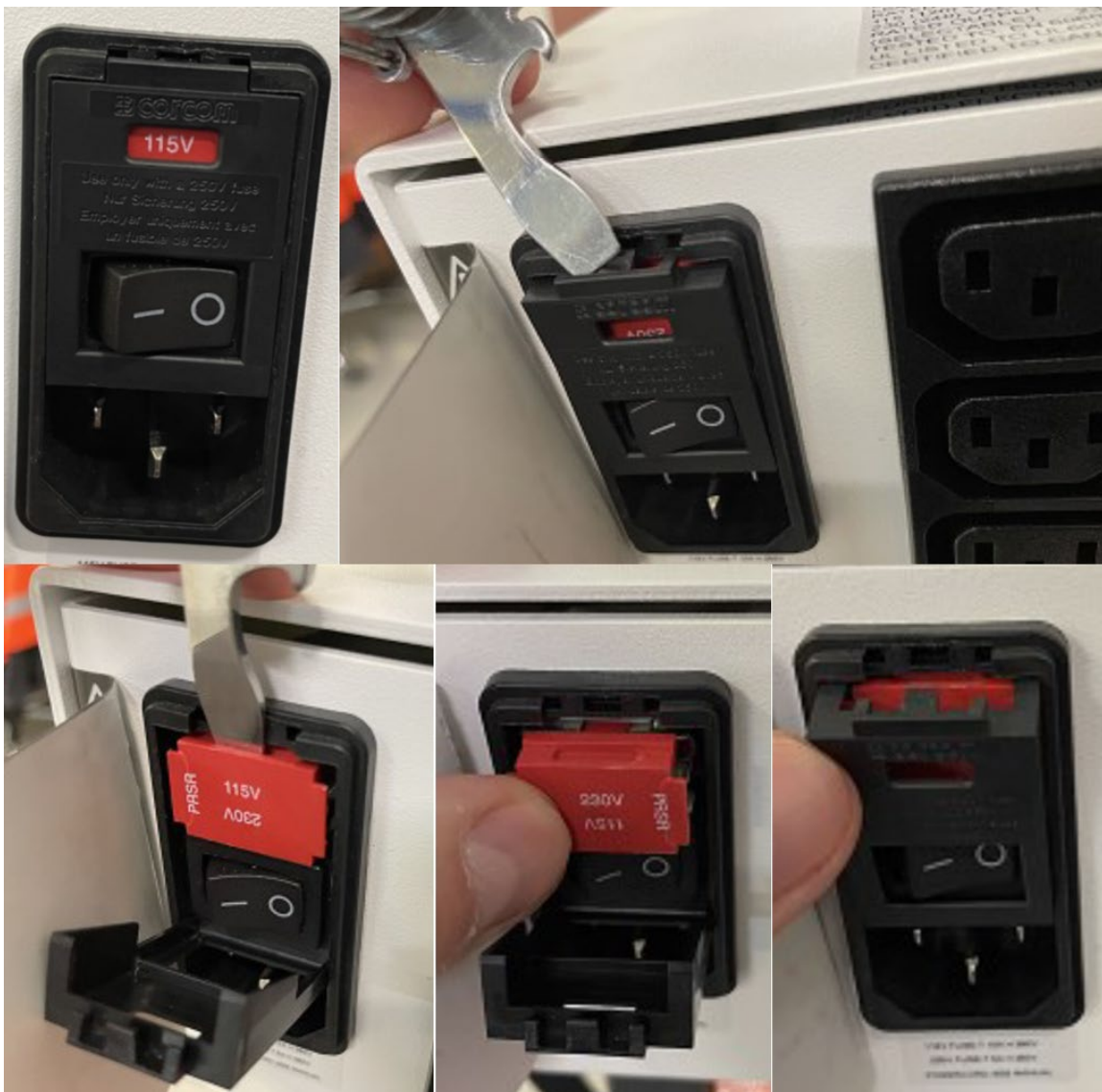
Figure 8: Changing input voltage setting of the Isolation Transformer
