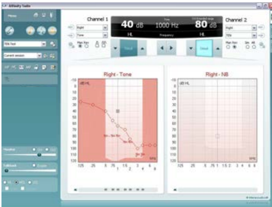
Figure 4. Screen shot from the Affinity 2.0 system. The open circles show the audiometric (absolute) thresholds. The “TEN” symbols show masked thresholds measured for TEN with a level of 80 dB HL. The TEN(HL)-test criteria for a dead region are met at 1.5, 3, and 4 kHz. The result at 2 kHz is inconclusive, as the masked threshold is not 10 dB or more above the audiometric threshold. In such a case, the result at 2 kHz could be checked using a TEN level of 90 dB HL. Overall, the results suggest that this patient has a dead region extending from 1.5 kHz upwards.
