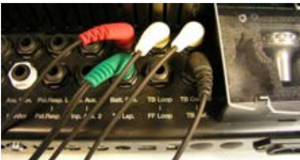
Figure 2: Cable placement on the Affinity/Equinox
